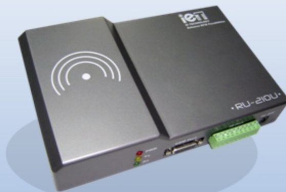
RU-210u: Desktop UHF RFID with USB Serial Interface
